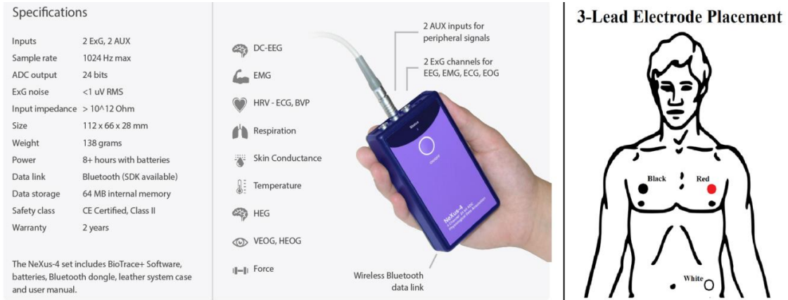
Figure 8. ECG Sensor System and Lead Placement.
