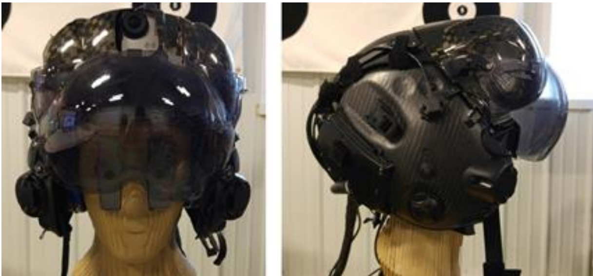
Figure 6. Representative 5th Generation HMD Used in Study.
